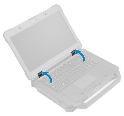
3. Place the brackets[1] and secure it using two  $^{1}M2.5*5^{1}$  on either sides [2].
