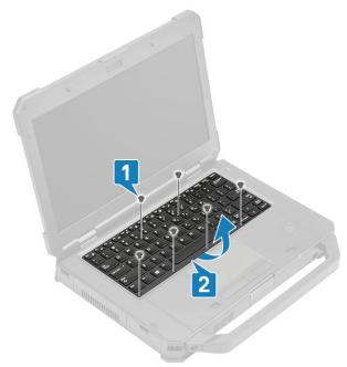
4. Slide the keyboard slightly [1] towards touch pad and flip it over inclined over the LCD panel [2].
