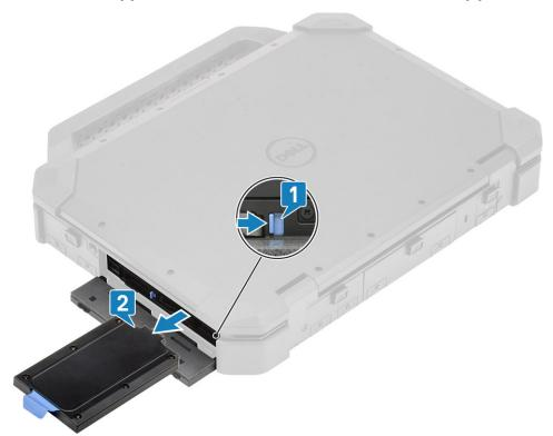
4. (i) NOTE: Depending on the configuration ordered the system may have a Hard Drive or a Solid State Drive in the carrier. The installation and removal procedure remains same.
