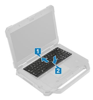
**6.** Install the six  $^{1}M2.5*5^{1}$  screws on the keyboard to secure it to the computer.
